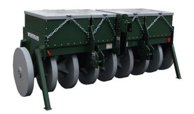
the outside wheels at the very edge of the machine, making it much easier to get a tight pack right up to the trench wall. The Weaverline Silage Packer is an efficient and very effective packing machine that will help to get consistent density numbers from top to bottom and wall to wall in your trench.
