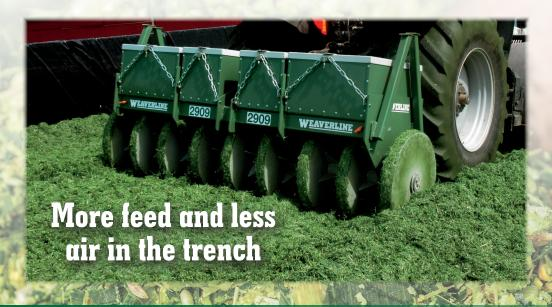
The Weaverline 2900 series Silage Packers are built to help you pack faster and better. With heavier wheels, no lip on the rim, and lower boxes for less vision obstruction, the 2900 series packers take the advantages of previously designed Weaverline packers and bring it all together in a machine that helps you pack more effectively, which means more feed and less air in the trench.
