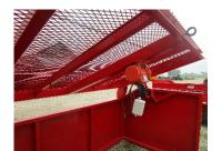
Oli vibrator 110V standard, purchaser to complete electrical wiring for their requirements and local codes. Can be operated with 110 extension cord, generator or inverter.
