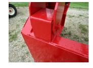
Screen hinge pins mounted in rubber blocks (use of isolating rubber mounts reduces vibration loss through main frame keeping as much vibration on the screen area as possible)
