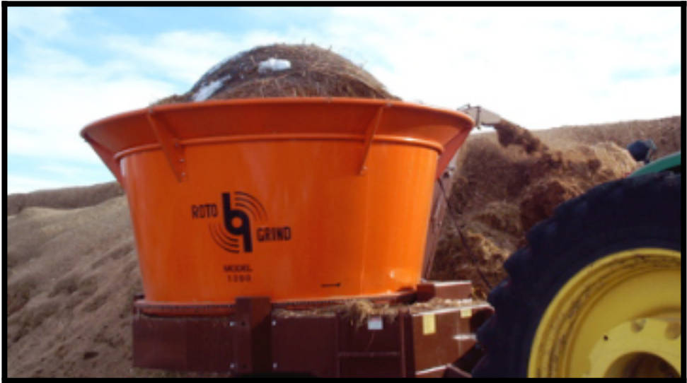
Model 1090 with Tub Flare Kit
