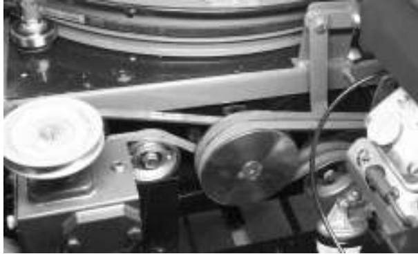
Figure 7 Rotor and Gear Box Drive Belt Installation
