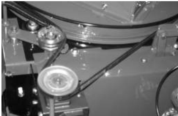
Figure 8 Hopper Belt Installation
