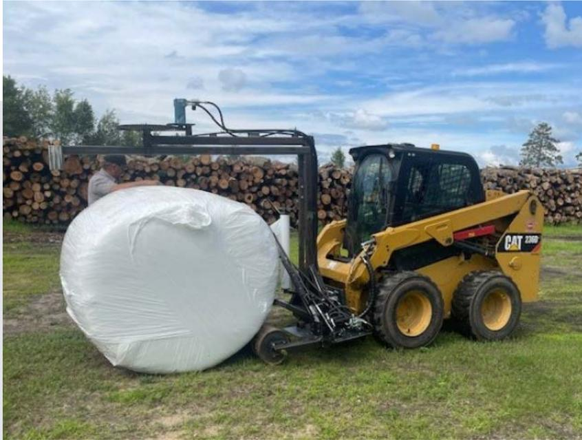
**The Bale Buddy 2000 was designed to allow hay to be baled while there is up to 60% moisture in the hay. When the weather is uncooperative, this will save time waiting for the hay to dry and product with less hay spoilage.**
