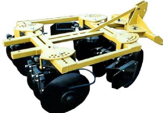
Shown w/ dirt diverters, cane deflectors, and mud scrapers
