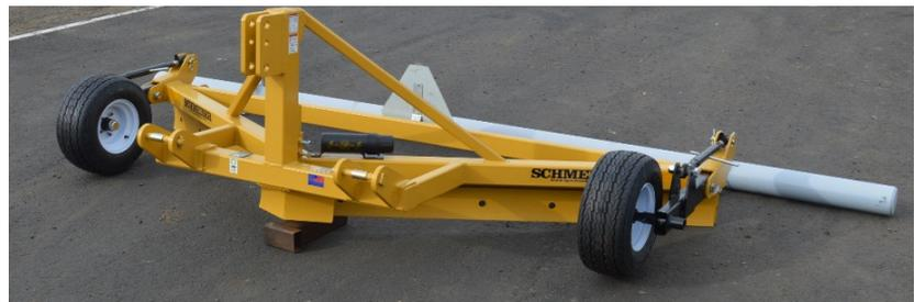
10 ft. wide main unit with turnbuckle adjustable gauge wheels, replaceable spindles, center buster and standard V-blade replacement blades (10 ft. rears). 14 ft. drag pipe for a smooth finish. Quick & easy post harvest clean up
