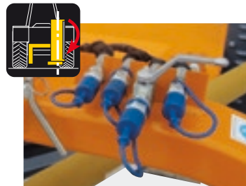
Hydraulic block tap of flail head during transport (no chains or holders).
