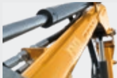
Circular section power arms High Torsion Resistance
