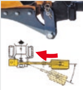
Mechanical breakaway (arm protection in case of obstacles)
