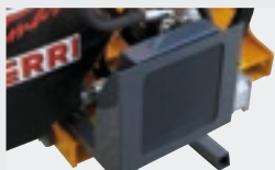
Oil cooler with thermostat
