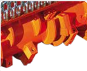
Apeiron rotor with fixed tools and tungsten carbide inserts with steel profiles.
