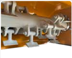
Rotor with unidirectional hammer blades.
