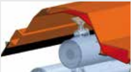
Inner lining for complete protection of the frame.
