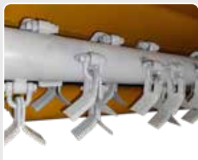
Rotor with articulated "Y" flails
