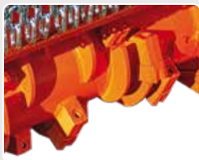
Apeiron rotor with fixed tools and tungsten carbide inserts with steel profile.
