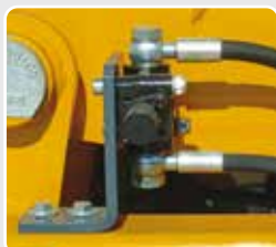
Single acting-double acting automatic switch.
