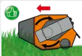
Self-leveling parallelogram device.
