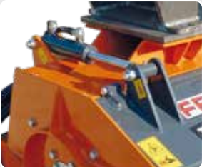
Hydraulic cylinder for the housing opening.
