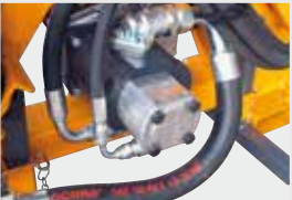
Group 3 cast iron hydraulic rotor pump
