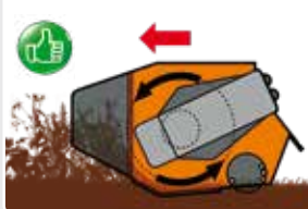
Rotor direction for grass and bushes.
