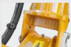
Drop forged parts for arm linkages
