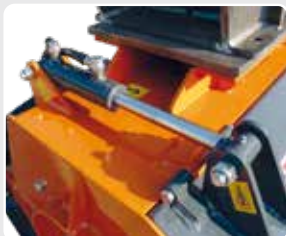
Hydraulic cylinder for the housing opening.
