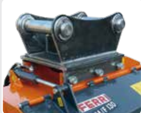
Dedicated attachmente linkage (recommended option see page. 82)
