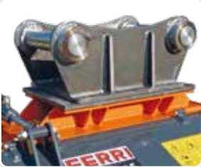
Dedicated attachmente linkage (recommended option see page. 82)
