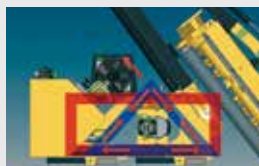
Frame "DELTA BOX" (forces shared and balanced)
