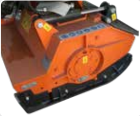
Adjustable skids with wear proof plates.
