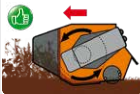
Rotor direction for grass and bushes.
