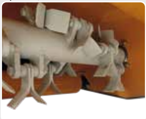
Rotor with multi-use and straight flails.
