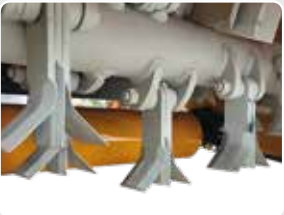
Rotor with multi-use and straight flails.
