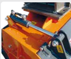
Hydraulic cylinder for the housing opening.
