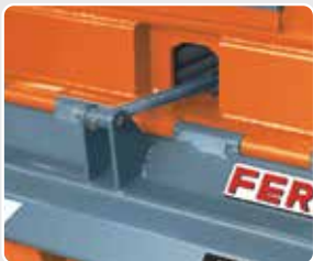
Hydraulic cylinder for the housing opening.
