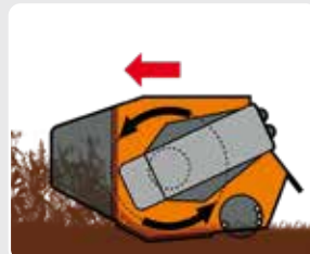
Rotor direction for grass and bushes.
