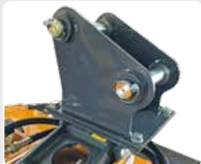
Dedicated attachment linkage (recommended option).
