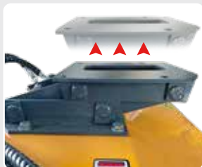
Self-leveling parallelogram device (optional).
