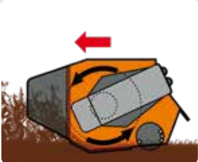
Rotor direction for grass and bushes.
