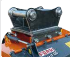
Dedicated attachmente linkage (recommended option see page. 82)
