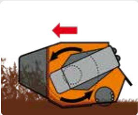
Rotor direction for grass and bushes.
