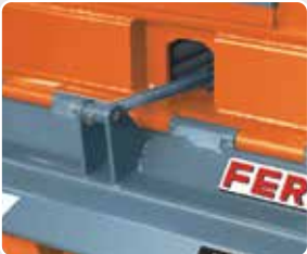
Hydraulic cylinder for the housing opening.
