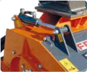
Hydraulic cylinder for the housing opening.
