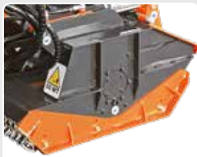
Hydraulic cylinder for the housing opening.
