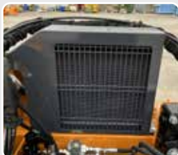
Oil cooler with thermo- stat.
