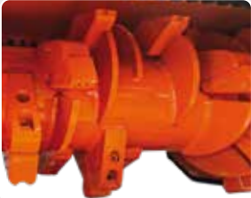
Apeiron rotor with fixed tools and tungsten carbide inserts with steel profiles.
