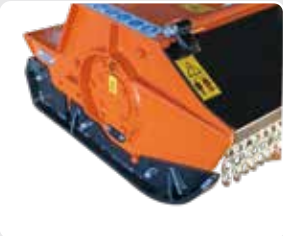
Adjustable skids with wear proof plates.
