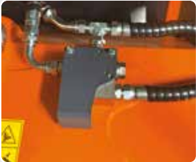
Calibrated steel adjusting valve.
