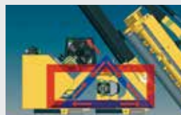
Frame "DELTA BOX" (forces shared and balanced)
