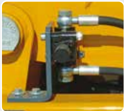
Single acting-double acting automatic switch.
