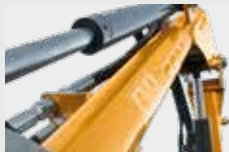
Circular section power arms High Torsion Resistance
