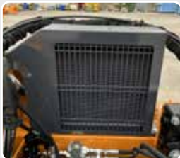
Oil cooler with thermostat.
