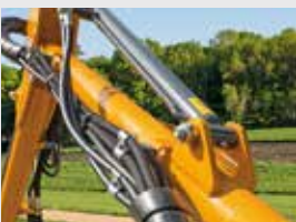
Arms with circular section H.T.R. (High Torsion Resistance).
