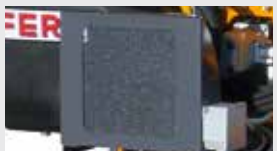
Oil cooler with thermostat (optional)
