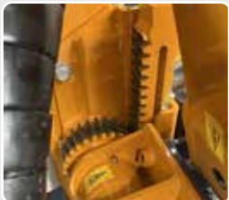
Rear mounted flailhead with rack and pignon gear to ensure the most precise cutting position.
