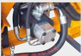
Group 3 cast iron hydraulic rotor pump
