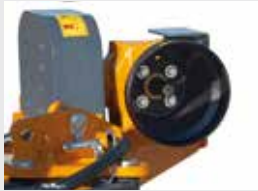
Gearbox external to the drive housing.
