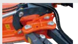
Rotation joint on self lubricating bushing.
