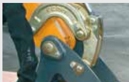
Drop forged lever for flail head rotation
