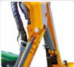
Hydraulic breakaway on second arm with accumulator controlled autoreset facility.
