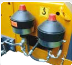
Lift float nitrogen accumulator.
