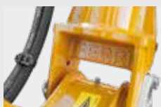
Drop forged parts for arm linkages
