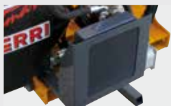
Oil cooler with thermostat
