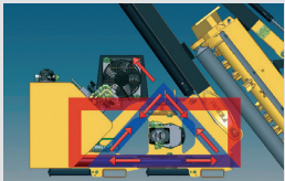
Frame "DELTA BOX" (forces shared and balanced)
