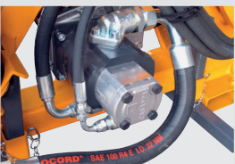
Group 3 cast iron hydraulic rotor pump
