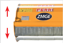
Floating frame following the ground contours
