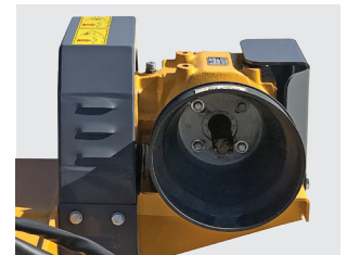
Gearbox unit outside the transmission cover
