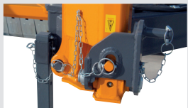
Floating frame following the ground contours.
