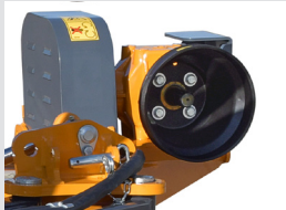
Gearbox external to the drive housing.
