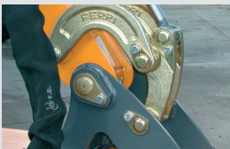
Drop forged lever for flail head rotation
