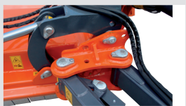
Rotation joint on self lubricating bushing.
