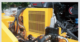
Oil cooler with thermostat
