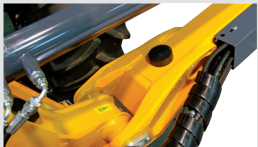
Frame "DELTA BOX" (forces shared and balanced)
