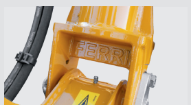
Drop forged parts for arm linkages
