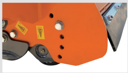
Rear adjustable roller 6 1/2"
