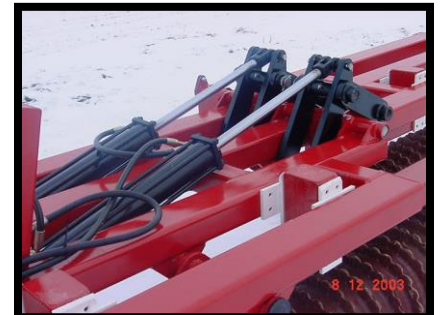
3 beam outerwing section w/ two cylinders, each packer gang oscillates on centre pin and plastic wear plates
