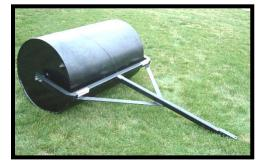
The drum is made from tubular steel 30" in diameter and 3/8" thick. The end plates are 10-gauge steel with 1" bearing on the standard roller. The Extra Heavy-Duty version uses  $\frac{1}{4}$ " steel with 1  $\frac{3}{4}$ " pillow block bearings.
