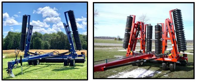
Flex packers are available in a 3-section configuration for widths of 21' to 32' (shown on left). Packers 33' to 50' are built on a 5-section frame (shown right). The balanced frame design minimizes tongue weight.
