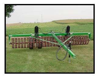
Match tillage or planting equipment with adjustable frame width ranging 9' to 15', and rigid frame on 3' to 6' and 16' models. Big Jim Packers are available in Red, Green, and Blue frame colours.
