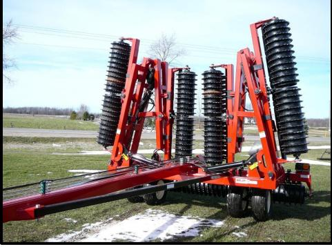
The Superflex concept has proven to be the most revolutionary design in packers for years. The independent floating design lets each section follow the contour of the soil giving more effective wheel to soil contact. The design also allows each section to independently float over obstacles such as stones without placing excessive weight on the gang causing wheel, shaft or bearing damage.
