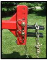
The adjustable hitch clevis has a wide range of settings to accommodate a variety of tractor drawbar heights.
