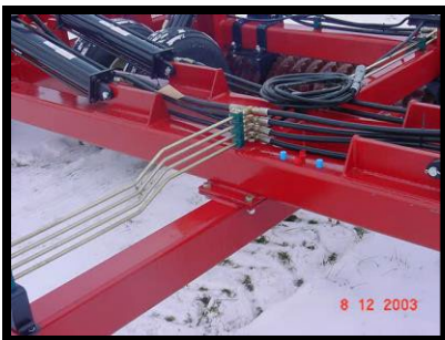
All plumbing neatly arranged and tied in place
