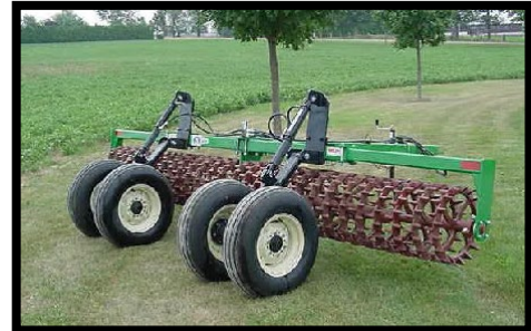
Shown with Dual Wheel Transport Kit
