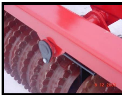
Rugged 1 3/4" hinge pins, securely fastened
