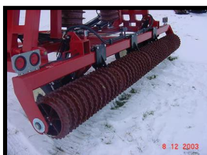
5 bearing main frame section, lights & reflectors standard
