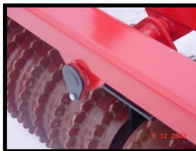
Rugged 1 3/4" hinge pins, securely fastened
