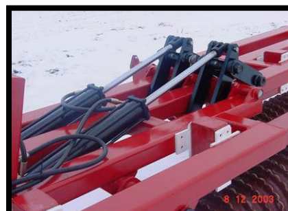
Rugged 4 beam main with section with two cylinders
