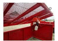
Oli vibrator 110V standard, purchaser to complete electrical wiring for their requirements and local codes. Can be operated with 110 extension cord, generator or inverter.
