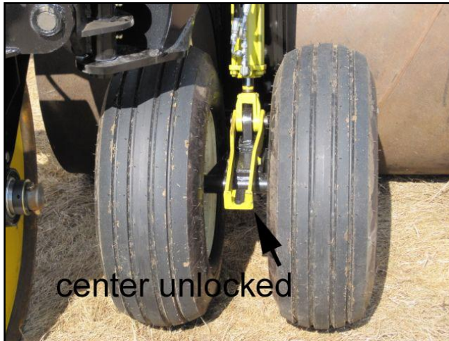
FIGURE 12 CENTER WHEEL UNLOCKED FOR FIELD
