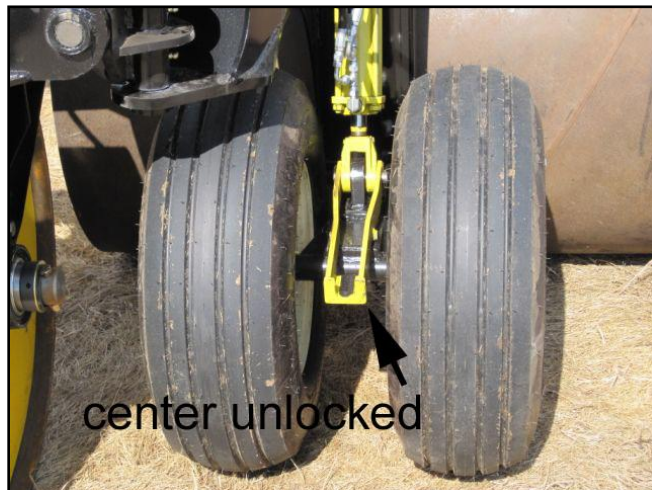
FIGURE 19 CENTER WHEEL UNLOCKED FOR FIELD
