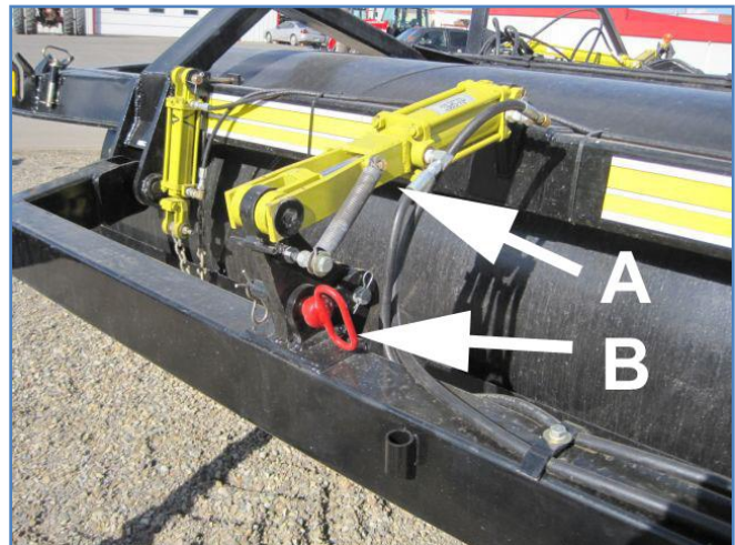
FIGURE 22 LOCKED FOR ROAD TRANSPORT
