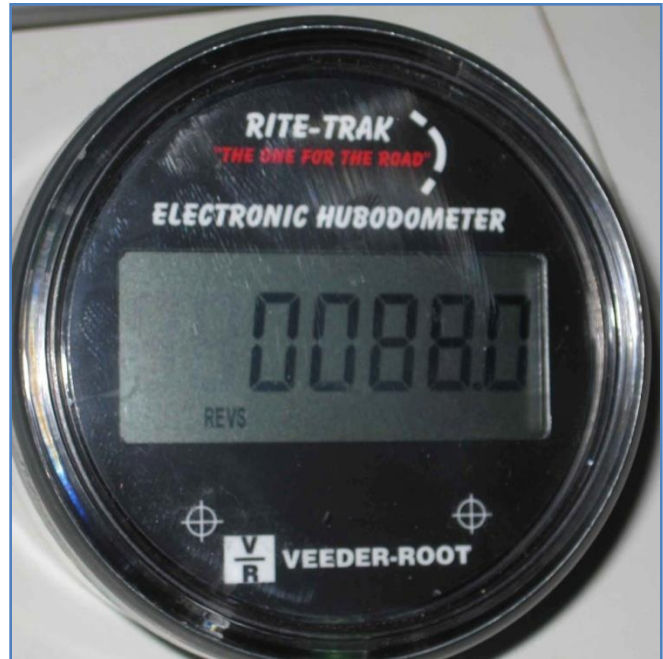
FIGURE 26 CALIBRATING "REVS" FOR 45
