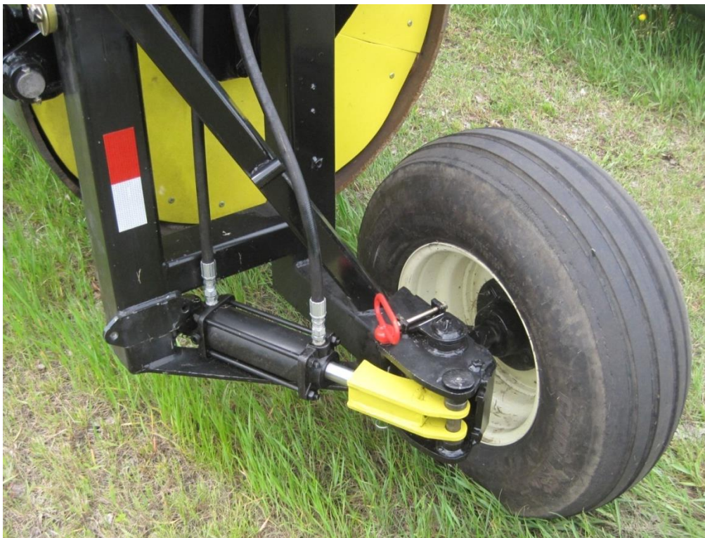
FIGURE 30 EASIFOLD WHEEL - HYDRAULIC TURN – NOT POWERFOLD-- LOCKED
