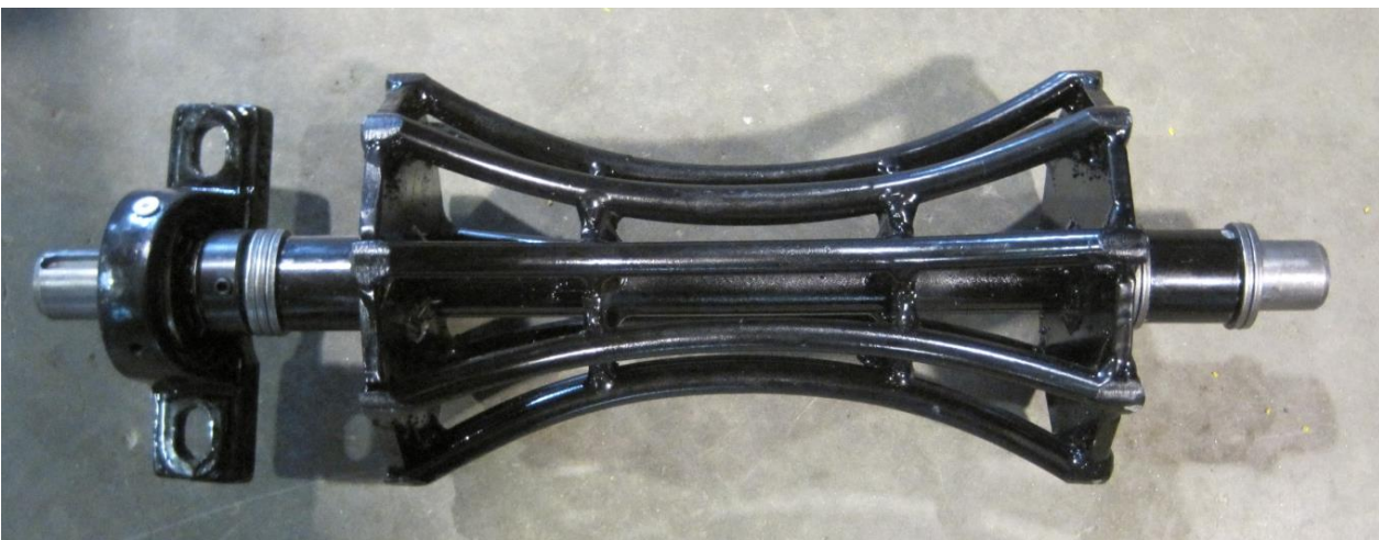
FIGURE 28 DRIVE SPINDLE WITH SPACERS & MACHINERY BUSHINGS TO SHIM TO CENTER
