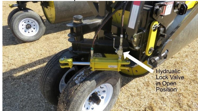
FIGURE 11 OUTER WHEEL UNLOCKED
