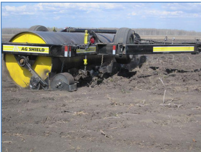
FIGURE 21 END GAUGING WHEEL SINKING INTO PLOUGHED GROUND
