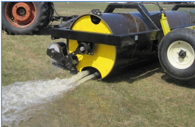
FIGURE 30 WATER DRAINING BY GRAVITY
