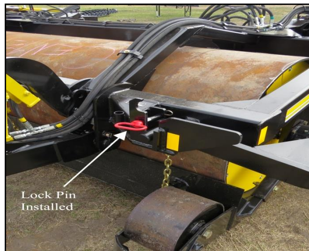
FIGURE 14 DIAGONAL PULL ARM LOCKED IN FIELD POSITION
