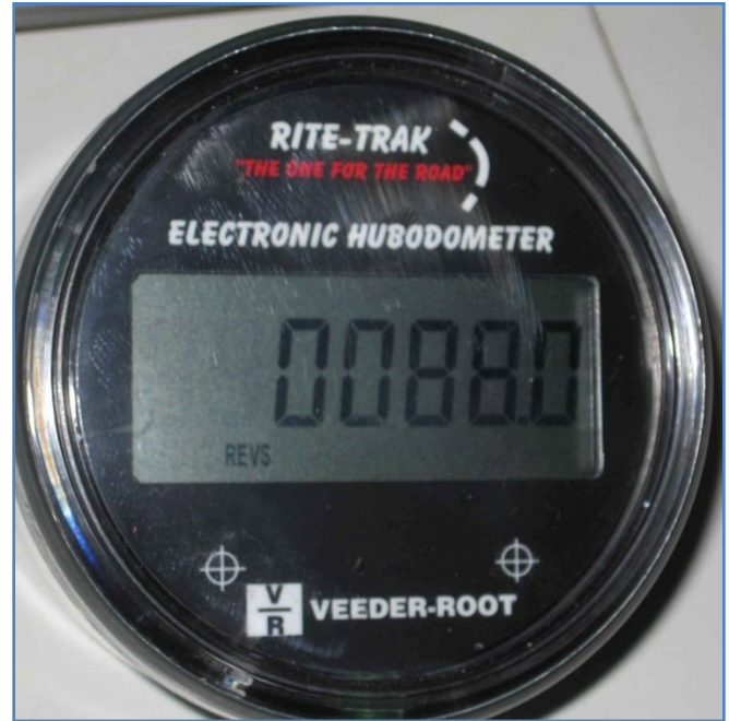
FIGURE 32 CALIBRATING "REVS" FOR 45
