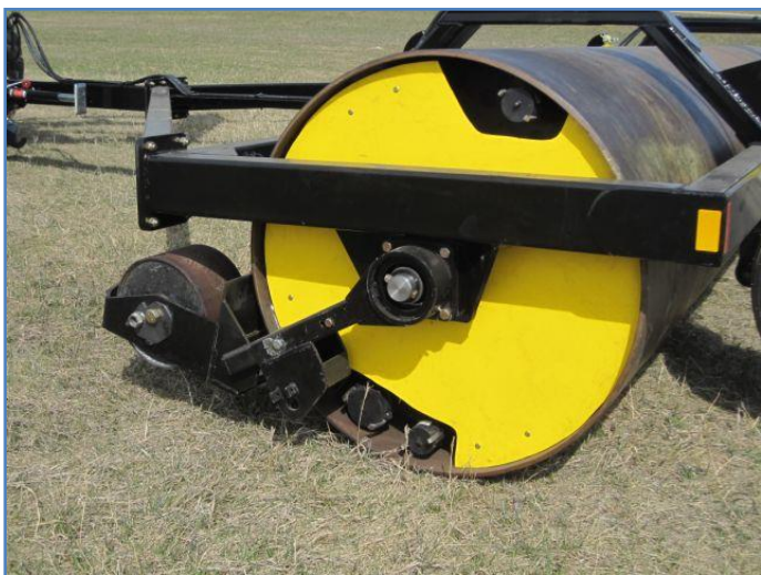
FIGURE 26 BLADE RAISED FOR TRANSPORT, CLEAR STONE, OR DUMP SOD
