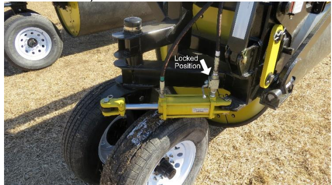
FIGURE 18 REAR WHEEL HYDRAULIC LOCK IN THE LOCKED POSITION
