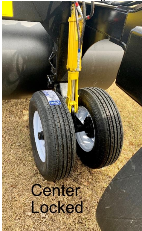
FIGURE 19 CENTER SECTION HYDRAULIC LOCK
