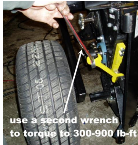
FIGURE 33 TIGHTEN LOCK NUT ON ROLER STOP
