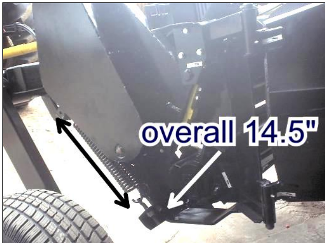
FIGURE 21 LH SPRING TENSION ADJUSTMENT
