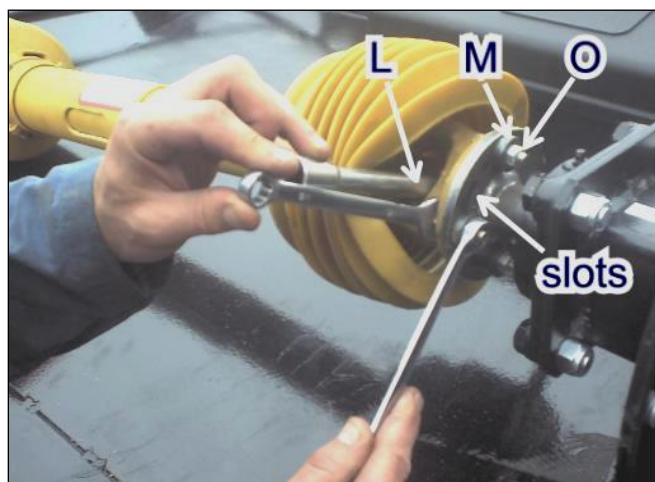
FIGURE 25 TIMING ADJUSTMENT ON SLOTS
