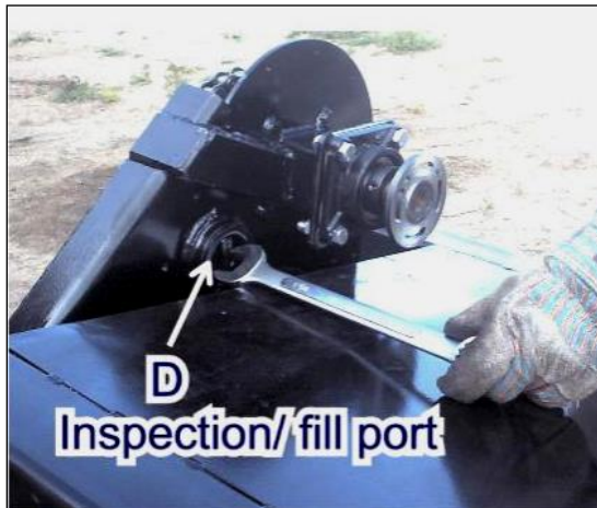
FIGURE 15 REMOVE INSPECTION FILL PLUG
