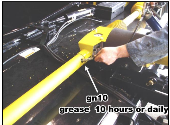
FIGURE 69 GREASE RH SLIP SHAFT GEARBOX
