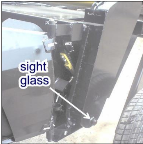
FIGURE 70 SIGHT GLASS LOW ON CASE
