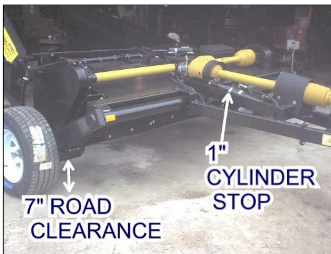
FIGURE 10 TRANSPORT LOCK- CYLINDER STOP
