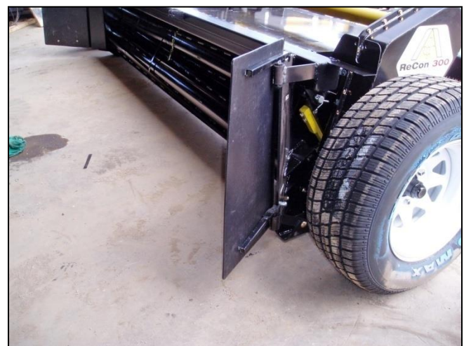
FIGURE 52 RIGHT WHEEL GUARD INSTALLED
