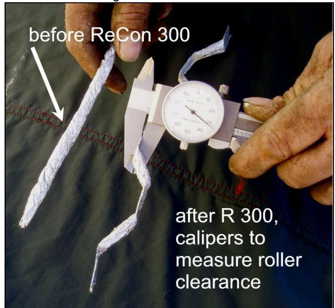
FIGURE 28 TIN FOIL TUBES BEFORE AND AFTER CRIMPING
