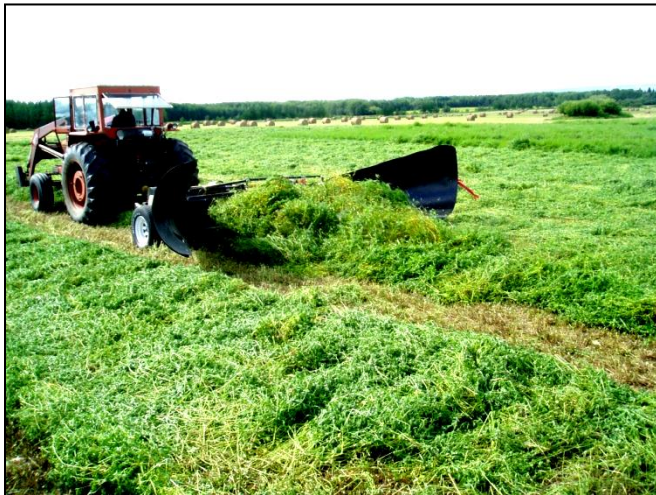
FIGURE 54 ALFALFA TO 11 FT WIDE WITH FIN KIT
