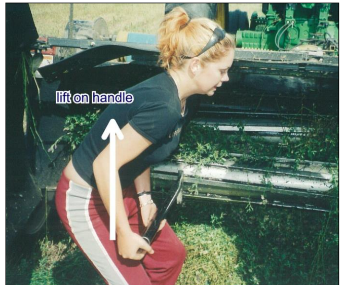
FIGURE 22 REVERSING ROLLER TO CLEAR WAD
