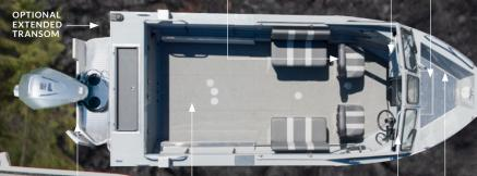
ALL-WELDED WINDSHIELD WELDED BOW WITH GRAB HANDLES FLOOR
