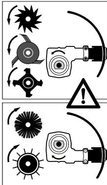
If you use metal tools, position the gearbox so that the axle is below the drive shaft.
