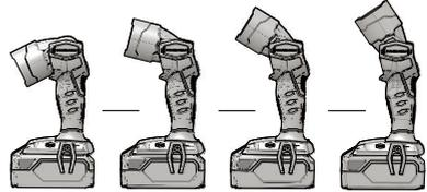
1. Turn the top head of the machine to adjust the light angle (0-135°).
