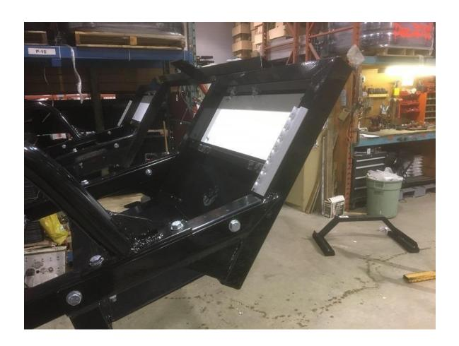
6. Now install the 2 side bars using the  $7 - 3 \frac{1}{3}$ " bolts per side.
