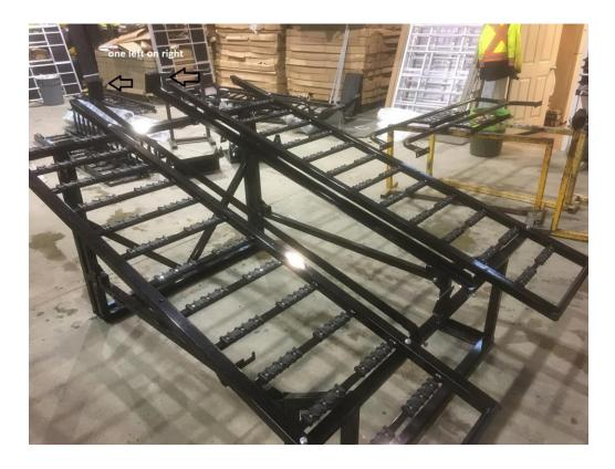
4. Bolt down the deck ramp sections to the leg assembles. Using the  $3\,1/4$ " bolts for the 4 outer holes then using the 5" bolt for the 4 inner holes, along with the washers, and Nyloc nuts.
