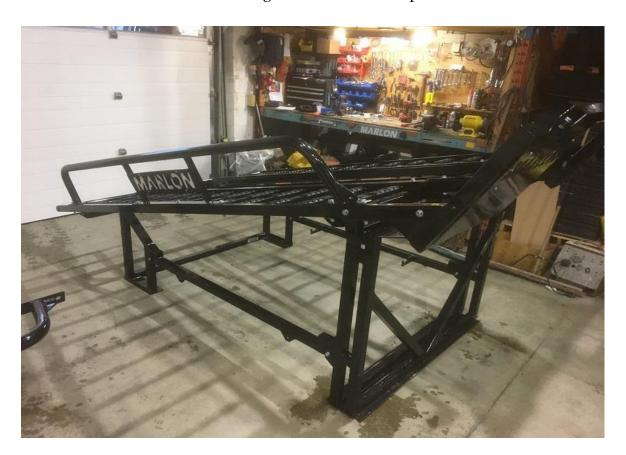
7. Now install the winch mount plate bar with  $2-3\frac{1}{4}$ " and  $2-5\frac{1}{2}$ " bolts
