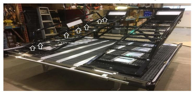
8. Now that all parts have been attached you can go ahead and tighten all nuts and bolts, starting from the deck mounting bolts and work your way up. All nuts should be torqued to 75 ft lbs.
