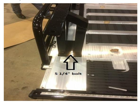
4. Attach the 2 main deck ramps to the front leg support with  $2 - 5\frac{1}{4}$  and  $2 - 3\frac{1}{4}$  bolts with washers and nyloc nuts (do not tighten).
