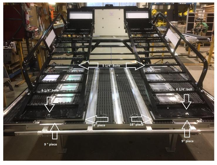
7. Attach side rail bars with  $14 - 3\frac{1}{4}$  bolts with washers and nyloc nuts (do not tighten).
