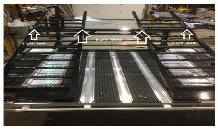
5. Slide on the front tire cradles and bolt in place with  $8 - 3\frac{1}{4}$  bolts (do not tighten). Then bolt on the front winch mount support with  $2 - 5\frac{1}{4}$  and  $2 - 3\frac{1}{4}$  bolts (do not tighten).
