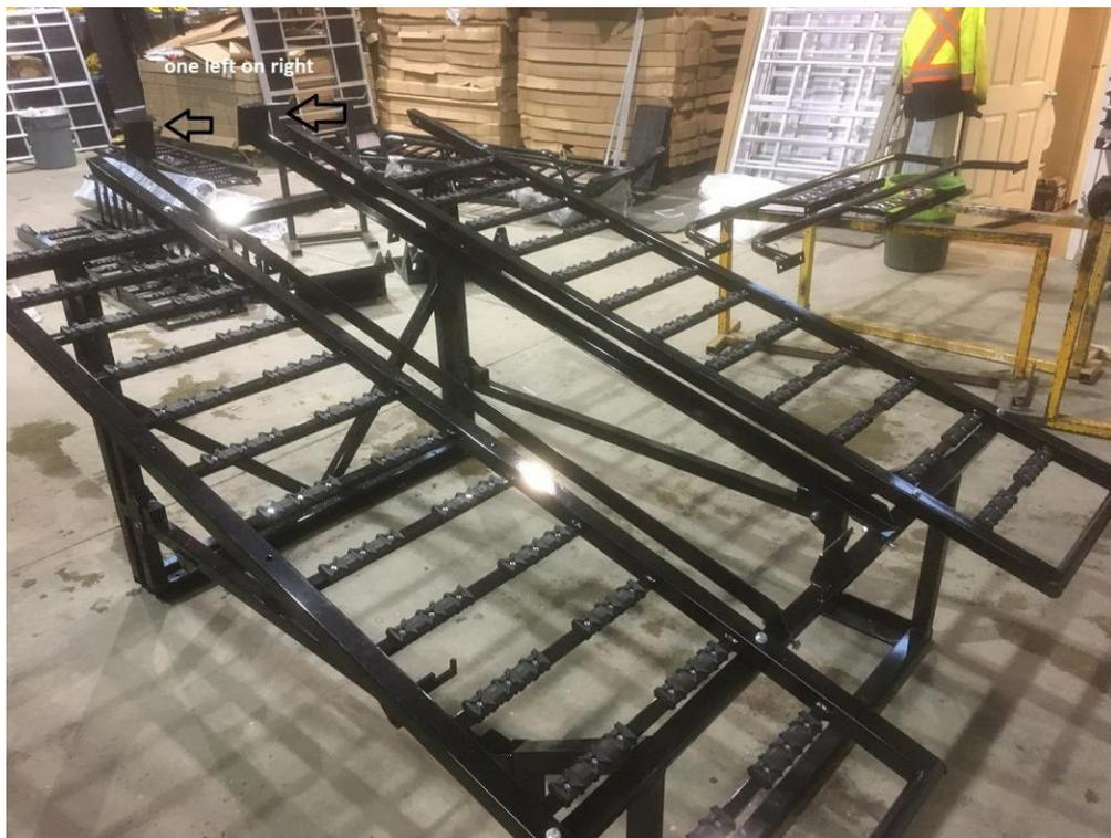
4. Bolt down the deck ramp sections to the leg assemblies. Using the 3 1/4" bolts for the 4 outer holes then using the 5" bolt for the 4 inner holes, along with the washers, and Nyloc nuts.
