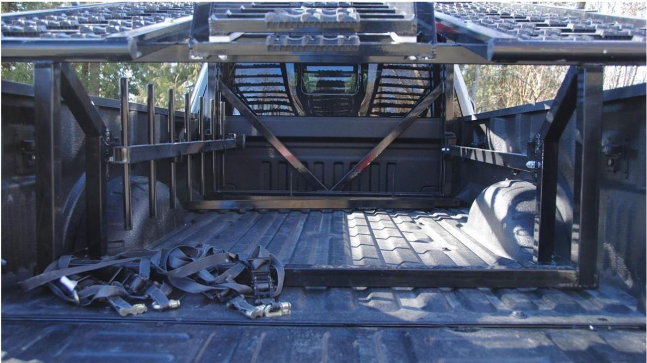
4. Drill a pilot hole through the center of the deck leg mounting hole, and the truck box – **be careful to not drill through any fuel lines.**
