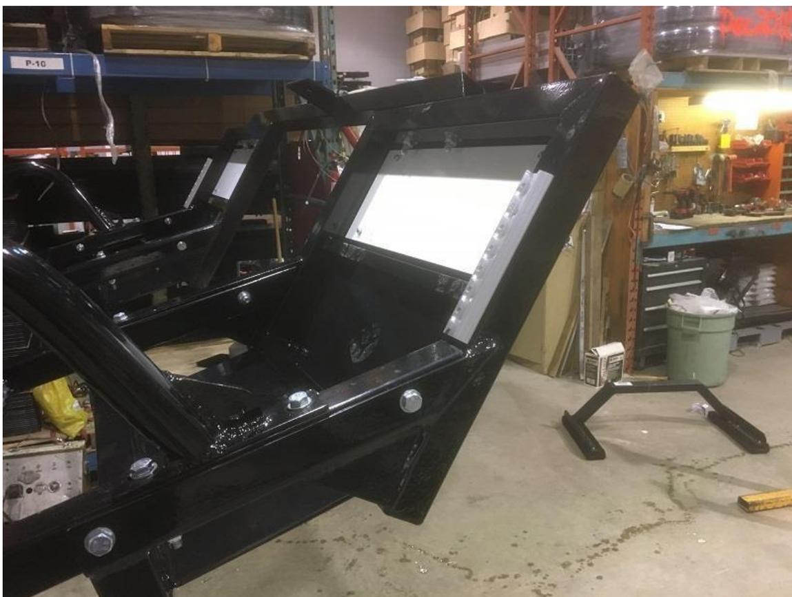
6. Now install the 2 side bars using the 7 – 3 1/3" bolts per side.
