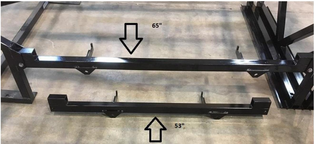
3. Bolt in the centers brace that supports the ramps with 3 1/4" bolt, washers and Nyloc nuts.
