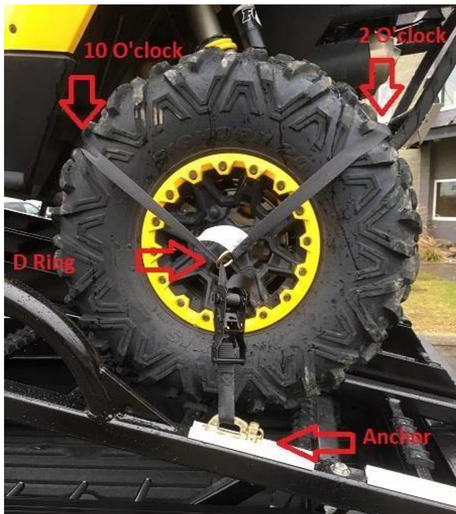
14. Repeat steps 12 and 13 on the remaining 3 tires. (remember to install the spring pin when using the movable ladder, this is imperative to the strength of the mounting positions)
