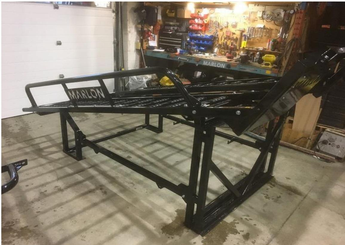
7. Now install the winch mount plate bar with 2 – 3 1/4" and 2 – 5 1/2" bolts
