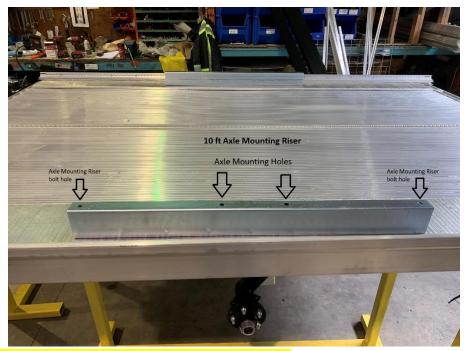
Note the axle mounting riser for the 10' (108 cm) has only one set of axle mounting holes. (See picture above.)
