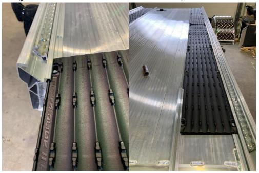
2. Rivet the extrusion down 1" from each end. Then staring at the back of the trailer at 30" then 70", then 110" (143" on the 12 ft) for a total of 5 rivets per length of extrusion. Then rivet the end of the front and rear glide as per picture below, it is not necessary to rivet any of the middle 2 glides.
