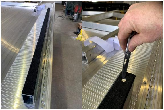
2. Bolt the axle mounting riser to the trailer frame with the adhesive barrier side up so that it contacts the frame. Use 200 x 10mm bolts, washers, and nylocks. Torque to 75 ft/lbs of pressure.
