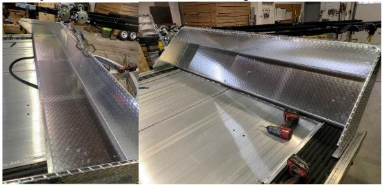
2. Position the shield over the leading edge of the trailer. Center it between the siderails and forward so that the leading edge of the trailer is inline with the bottom bend on the shield. (See pic below.)
