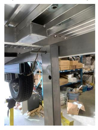
5. Swing the tongue up into place and install the tilt lock out bolts.
