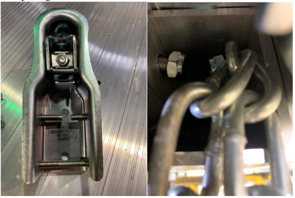
7. Install the tongue clamp bolt and brace. This is the 270 x 12.5 tongue clamp bolt with the 2 bends.
