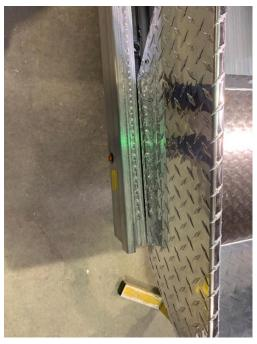
3. Screw down the shield with the self-tapping stainless steel screws, there are 15 predrilled holes to use as guides.
