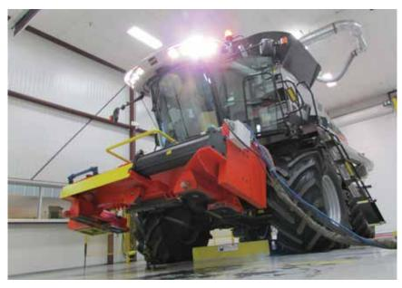
The dyno bay features a jounce test that rocks the combine back and forth, checks all its sensors, electrical, hydraulics and diagnostic systems and provides a thorough break-in of transmission and final drives. Even the cab lighting is adjusted to the proper angle. Over 120 areas are checked and monitored before a Gleaner goes to post-production inspection.
