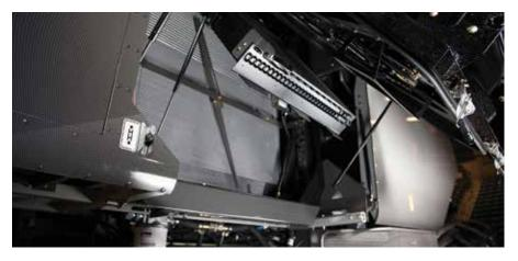
The entire rotary screen box and coolers pivot out for easy service inspection. Exclusive SmartCooling<sup>™</sup> eliminates the need for daily cleaning of the radiator, coolers and rotary screen even in heaviest soybean dust and chaff.
