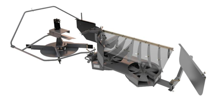
The S8 Super Series features a completely redesigned 2-speed chopper for greater residue chopping demands when required. For high speed chopping, the smaller 7 ½-inch chopper drum features 24 knives, a 50% increase, for greater chopping and a 16% increase in speed to 3,250 rpm to create enough vacuum pressure to pull residue on through and keep the processor cage clean, optimizing processor performance.
