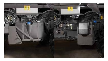
Gleaner S8 models feature a new integrated tool box located in the front of DEF tank for easy ground level access. The DEF tank support includes a pivoting feature that swings out and away from the machine for easy access to all the lower drives and drains for clean grain and tailings elevator troughs for improved serviceability.
