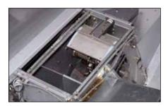
The Yield Sensor II measures the mass of grain flowing through the grain elevator.
