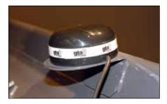
The DGPS antenna for the Fieldstar® II yieldmonitoring system receives its information from the WAAS Satellite System to pinpoint field location.
