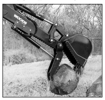
Figure 12. Thumb Operation
