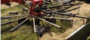
**LONG TINES** feature smooth front surfaces for long life and smooth crop release, creating a clean, uniform windrow. Our tine design also allows easy individual replacement of the tines, making it easier to maintain.
