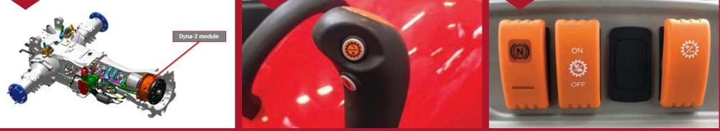
The Speed Matching provides the automatic selection of the appropriate Dyna-2 ratio when a gear change has been made. The speed matching feature minimizes driver effort and maximizes journey times.
