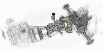
The left-hand Power Control lever provides convenient three-in-one, simple operation through the state-of-the-art transmission. Operators can shuttle between forward and reverse without clutching, making jobs that require frequent direction changes, like loader work, a breeze. Shuttle responsiveness can be modified by simply adjusting the comfort control dial.
