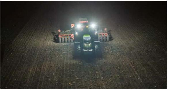
More light to work by – delivered by the 360° LED lighting concept on the Fendt 700 Vario. Premium quality LED headlamps offer a wide view as well as increased safety on the road. They are especially bright yet low-impact and long lasting.
