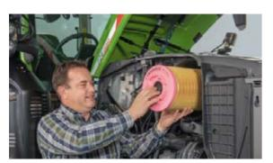
A swing-up bonnet and removable side panels provide excellent access to the engine compartment. This means you can quickly and easily remove the air filter.
