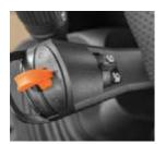
2 programmable lighting modes Use the switch on the reverse lever to quickly toggle between two stored lighting modes, including road and field mode.
