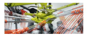
**3-D rotor suspension.** The gimbal suspension ensuring rotors adjust laterally and longitudinally to the ground contours independently from all tractor functions. This allows the LINER to deliver superior windrows in any conditions.
