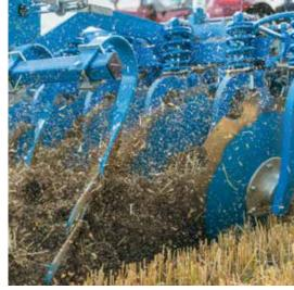
Compact disc harrows provided previously intense and homogeneous mixing of soil and organic matter to a depth of approximately 14 cm.
