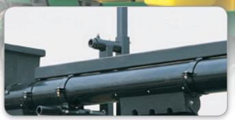
A steel mounting frame and 2" x 3" steel bracing keep the auger straight for longer life of all components. Arms on units for 16-row planters swing to accommodate flex-frame planters.
