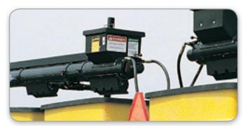
Powered by a reliable 6-cubic-inch hydraulic motor, the on/off control valve is conveniently positioned by the hopper for easy, one-person operation. The motor performs best with 8 to 12 gpm flow. An optional control valve package for adjustable hydraulic speeds is available.
