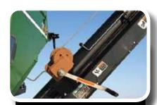
Winch system for easily moving conveyor from storage to working positions
