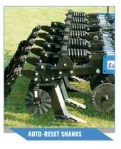
Shear-bolt trip mechanism features 9,000 lbs. of shear pressure and can be used in lighter, rockfree soils.
