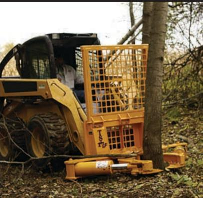
The powerful TS-17 tree shear is Fabrication S. Houle's rugged double bladed model. With this tree shear you can easily cut trees up to 17 inches in diameter, at ground level if needed. The replaceable and adjustable steel blades pivot on MOS-2 polyethylene bushings and all pivot points are greaseable. A shield provides increased protection for the hydraulic hoses. Designed for skid steer loaders and telehandlers.
