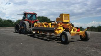
The DRR-30H is a double auger rock rake designed for major chores. With two 14' floating augers, the unit unfolds to an angle of 120 degrees to achieve a total working width of 27 feet. The unit has a 30 inch central area allowing the formation of a single rock swath. Hydraulic drive activated by tractor PTO, protected with overflow caution valve and cooled with thermostatic bypass valve. Comes with hydraulic depth control.
