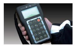
**CONVENIENT CONTROL.** A remote control allows operators to view engine parameters and change a variety of settings.
