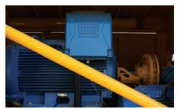
**ELECTRIC MOTORS.** The TG7000E is powered by two electric motors that deliver a combined 1000 hp (746 kW) to the mill. A separate 75 hp (56 kW) electric motor powers the pump for the hydraulic circuits, while a 2 hp (1.5 kW) electric motor powers the fan to cool the hydraulic system.
