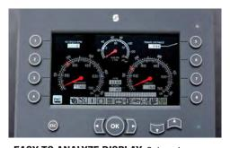
EASY TO ANALYZE DISPLAY. Onboard diagnostics include fault codes for enhanced serviceability and troubleshooting.
