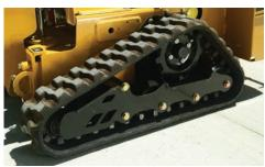
**DECREASE TURF DISTURBANCE.** Dual rubber tracks with a ground pressure of 3.7 psi (.3 bar) minimize disturbance and restoration to the jobsite while tackling tough ground conditions. This lightweight plow will also help save time with a 3.7 mph (6 km/h) transport speed.
