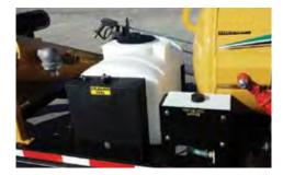
40 GALLON WATER TANK. Has 40 gal (151 L) of fresh water with 4 gpm (15 L/min) @ 3,000 psi water pump.
