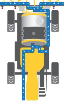
Rain, wind and a hundred other things can stop a job before it's done, letting residues settle in the plumbing. ClearFlow<sup>™</sup>, the industry's first full-recovery system, pushes unused product from the plumbing back into the tank, prior to a tank or boom rinse. Product goes back in the tank to be reagitated or off-loaded, minimizing waste and contamination. So you'll be confident plumbing and booms are clean.
