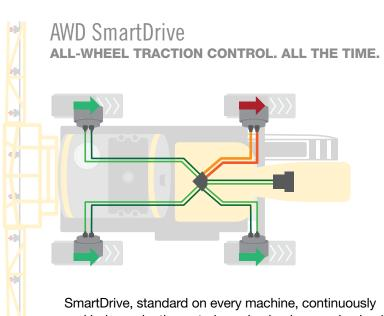
SmartDrive, standard on every machine, continuously and independently controls each wheel, so each wheel always gets all the torque it needs, when it needs it. Wheel slip is automatically countered by sending more power to the gripping wheels, while managing the slipping wheel to regain traction. The best part: you don't even have to tell it to do it.
