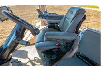
Help lessen operator fatigue with the optional deluxe vibration reduction system (VRS) vented leather seat with semi-active suspension.
