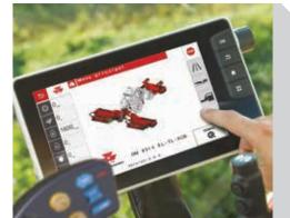
ISOBUS allows an implement manufacturer's control system to be displayed on the terminal screen, saving owners and operators time and money, with no need to install additional monitors in the cab.
