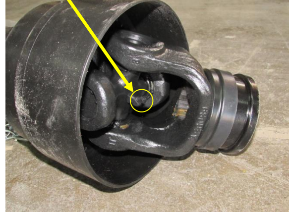
c. The two grease fittings on the safety shield and the inner portion of the PTO
