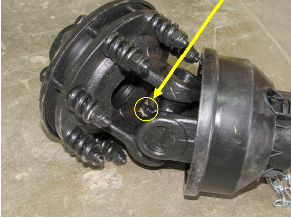
c. The two grease fittings on the safety shield and the inner portion of the PTO
