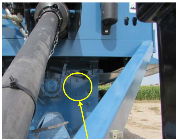
Front access door
