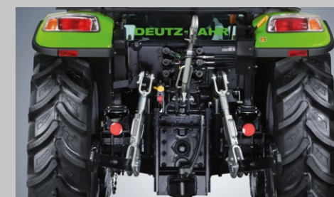
50 l/min hydraulic pump, up to three control valves, 3,500 kg rear power lift, 540/540ECO/1000 PTO.
