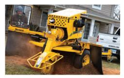
**FLOATATION TIRES.** This standard feature allows the weight of the machine to be dispersed over a larger area reducing the ground disturbance.
