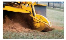
**AUTOSWEEP.** The patented AutoSweep<sup>®</sup> control system monitors engine speed and automatically adjusts cutter wheel sweep rate to maximize power to the cutter wheel while reducing engine stress.
