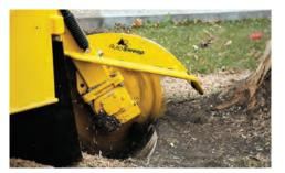
**SWING ARC.** The sweep arc measures 103" (261.6 cm). The below-ground cutting depth of 25" (63.5 cm) allows operators to cut even the largest stumps efficiently. The rear deck design allows for chip containment capacity of approximately 68 cu ft (1.9 cu/m).
