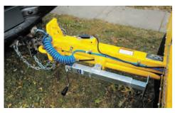
**TONGUE LENGTH.** A 60" (152.4 cm) tongue extension helps reduce the amount of repositioning needed on a jobsite.
