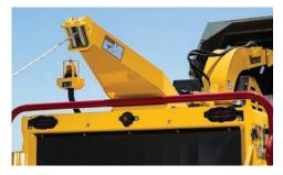
**EASILY LIFT HEAVY MATERIAL.** An optional winch allows operators to move large logs effortlessly. The 150' (45.7 m) winch line has 2000 lb (907.2 kg) pulling force and can automatically lift the log onto the feed table. With the chain choker detached it is also more easily attached to log than hook-on cable designs.
