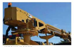
**HYDRAULIC BOOM.** Exclusive telescoping boom maintains hose length during extension and incorporates a remote-controlled hydraulic valve for vacuum shutoff. Available with manual or hydraulic rotation.
