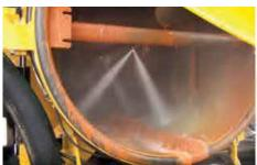
IN-TANK WASHDOWN. Delivers a highpressure water spray to the tank interior helping to simultaneously dump material and clean the inside of the tank. Minimizes cleanup time and helps remove difficult debris.
