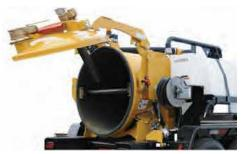
CAM-OVER REAR DOOR. Provides a 360-degree positive seal, even under reverse pressure without additional clamping requirements. The highly reliable cam-over door has no in-tank moving parts, so all maintenance is external.
